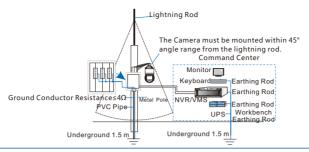
[Note]: If there is middleware installed, such as optical transceiver or anti-thunder device, the middlewareshould be well grounded and the camera should also be well grounded if the cable goes through the middleware.
