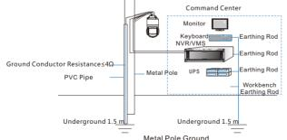
Metal pole with lightning rod applies inside PVC pipe to lead ground wire, and the PVC pipe should keep an insulation distance from the inner wall of metal pole as far as possible, as the picture shows.
